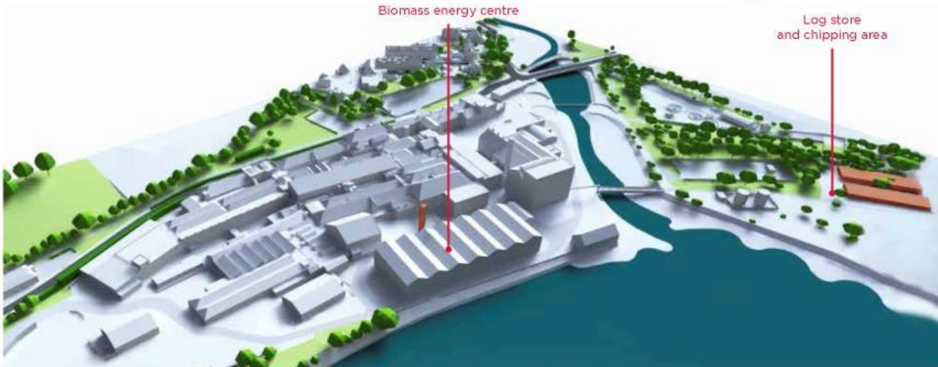
3D view of proposed biomass energy centre site - the biomass energy generating process will be contained within the existing Pulp Shed, and a new flue is to be constructed on the western side of the shed
